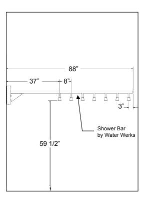
\* Adequate reinforcement backing is required. Use of metal stud is not sufficient reinforcement and is not recommended. Use of wooded stud is acceptable or equivalent. Failure to provide adequate reinforcement will result in damage to the Ditto Vichy Shower and may cause bodily harm and serious injury.
